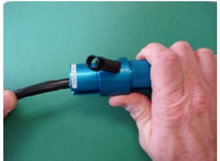
3) Locate the grounding clip. **Make sure that it is detached from the grounding cable and has not been deformed.** Open the clip slightly and snap it onto the cable.
