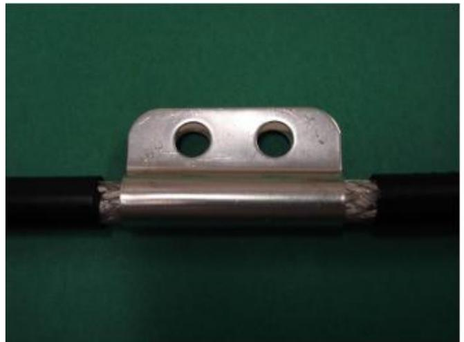
5) Attach the grounding cable to the grounding clip using the 1/4" brass nuts and lock washers. Tighten the nuts using a 7/16" open end wrench.
