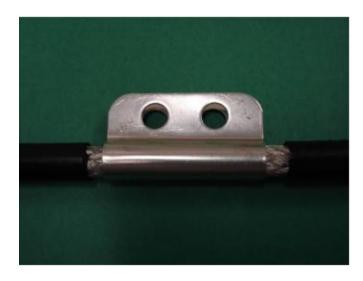
5) Attach the grounding cable to the grounding clip using the ½" brass nuts and lock washers. Tighten the nuts using a 7/16" open end wrench.
