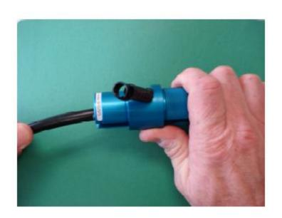
3) Locate the grounding clip. Make sure that it is detached from the grounding cable and has not been deformed. Open the clip slightly and snap it onto the cable.
